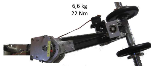
Fig. 6. The final MACCEPA-based SPEA with cylindrical cam mechanism. On the left the motor and cylindrical cam mechanism and self-closing guides. On the right the pretensioning mechanism for variable stiffness.
