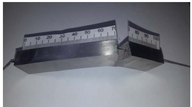
Figure 8. The location of the fatigue crack is measured to be 71 mm away from outer roller 1.
