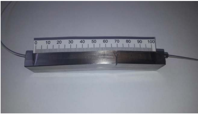
Figure 12. After approximately 7.20 Mcycles, the fatigue crack was clearly visible and located at 70 mm from outer roller 1.
