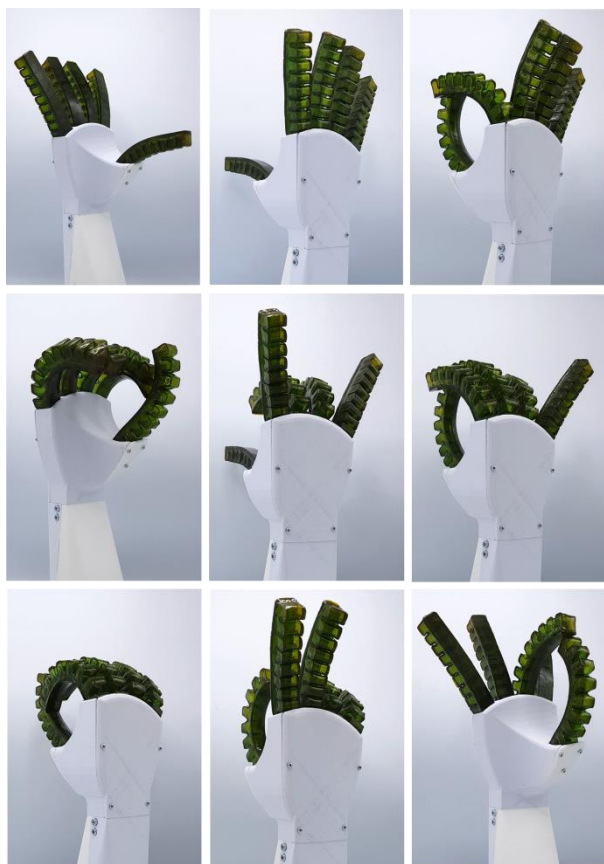
Fig. 7: The five BSPAs can function together in a soft hand that illustrates the potential of autonomously healable DA materials for social soft robotic applications. The fingers can be controlled separately, which allows the hand to make simple hand gestures. 2
