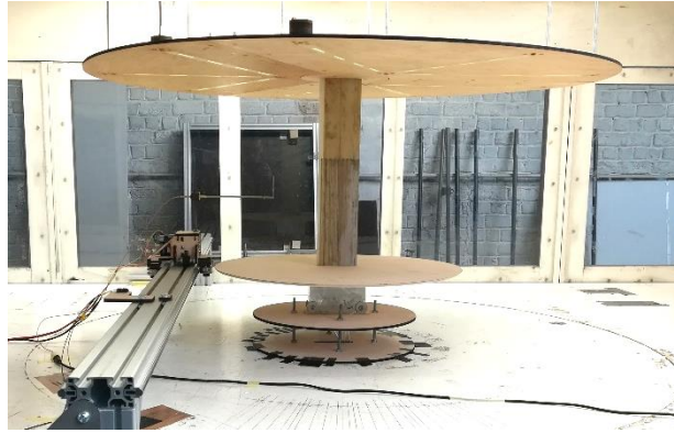
Fig. 5. Airfoil model overview, with end plates and traversing system.
