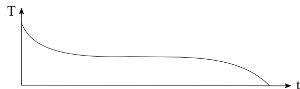
Figure 30: Approximated representation of the torque-time curve of a Twisted Elastic CTM.
